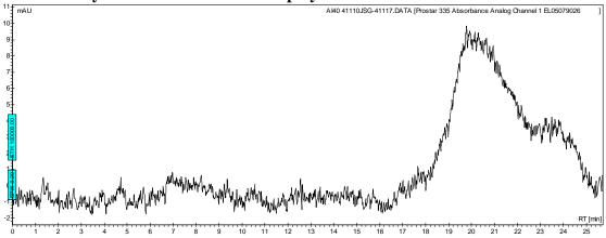
Analysis Method: Varian Prostar system with 1 ml/min DCM flow across two Phenogel  $5\mu m$  columns and one PLgel Resipore column (Agilent). Detection via UV/Vis, calibrated against polystyrene standards.
