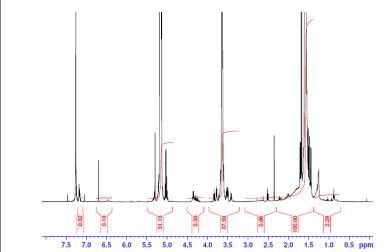
H-NMR Spectrum of PLLA-PEG-Mal copolymers in CDCl3 (Varian Inova 500 MHz instrument),
